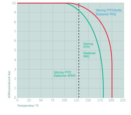
These limits apply to the intended use. Process variables and characteristics of the medium can influence the values of the diagram. Temperatures below 0 °C upon request.
